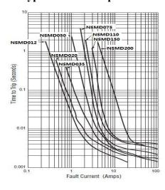
◆ Time to Trip curves represent typical performance of a device in a simulated application environment. Actual performance in specific customer applications may differ from these values due to the influence of other variables.
